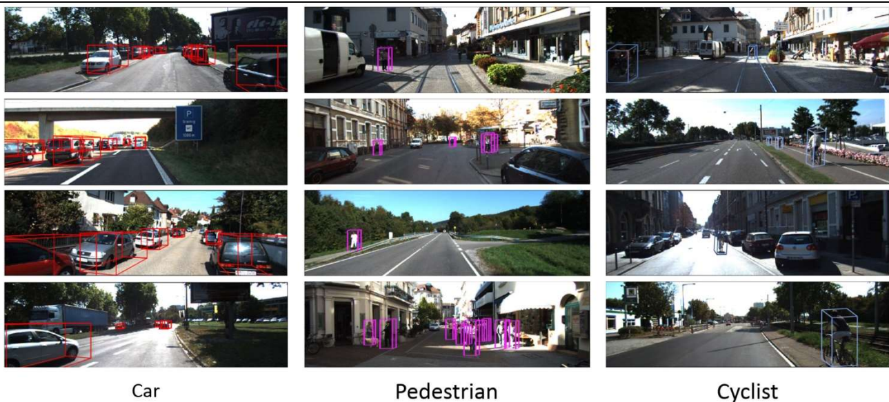
Figure 6. Qualitative results. 3D boxes detected with LiDAR are projected onto the RGB images.
