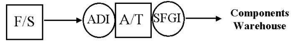
Figure 1: Material flow for 2 nodes: F/S stands for Fab/Sort, A/T stands for Assembly/Test
