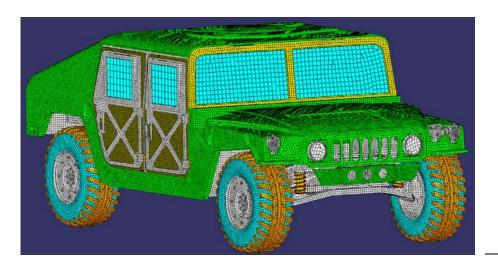
Figure 1. Geometrical meshed model for HMMWV vehicle used in the present work
