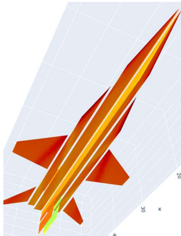
FIGURE 8 – North American X-15 VORLAX model used to estimate aerodynamics.
