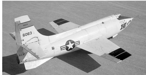
FIGURE 40 – Retrofitted Bell X-1E airframe with enlarged vertical tail surfaces (note a pair of Ventral fins) [79]
