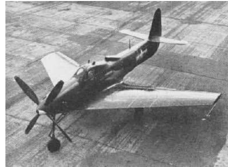
FIGURE 27 – Bell L-39-2 Swept Wing Testbed Aircraft with “Circular Arc” Airfoil Wing [53]
