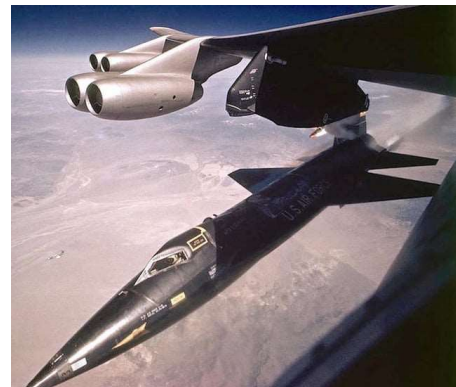
Fig. 23 X-15 immediately after being airdropped from the wing of a B-52 Stratofortress. All missions occurred within the designated test corridor near Edwards AFB, even when the X-15 was in outer space. It would usually travel a terrain distance of 200-300 miles for a mission.
