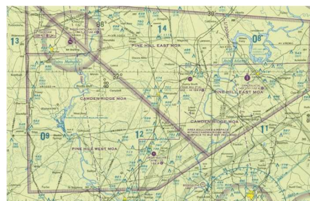
Fig. 17 Several cohesive MOAs. Aircraft flying through these must acknowledge them with caution and will be escorted away during testing and training procedures.
