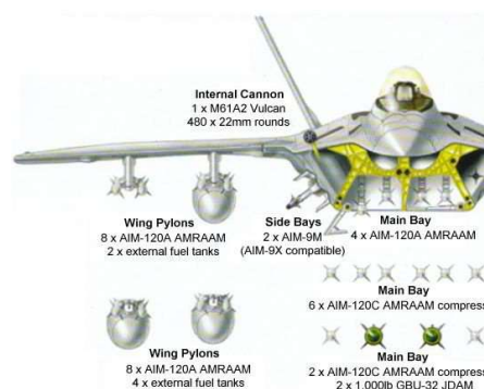
Fig. 9 Example of internal and external weaponry on an F-22 Raptor.
