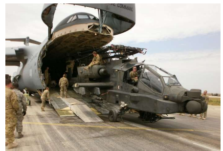
Fig. 7 AH-64 Apache helicopter inside a C-5 Galaxy. Different requirements drive different designs. Sometimes they are even transporting other aircraft.
