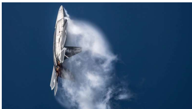
Fig. 5 F-22 Raptor executing a 'Power Loop' maneuver. The aircraft experiences high structural stress and load factors during sharp maneuvers.
