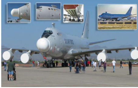
Fig. 10 Boeing YAL-1 with laser integrated testbed. It successfully destroyed an ICBM in 2010 and was eventually scrapped. Its technology, test data, and applicable regulations will be very valuable for years to come.
