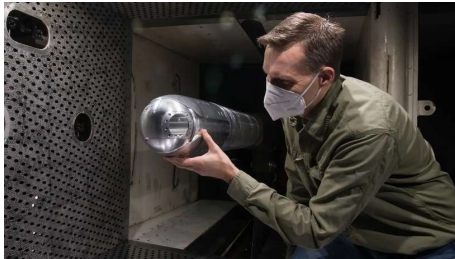
Fig. 11 Air Force engineer testing a laser weapon in a wind tunnel. The laser is to be installed on fighter jets.
