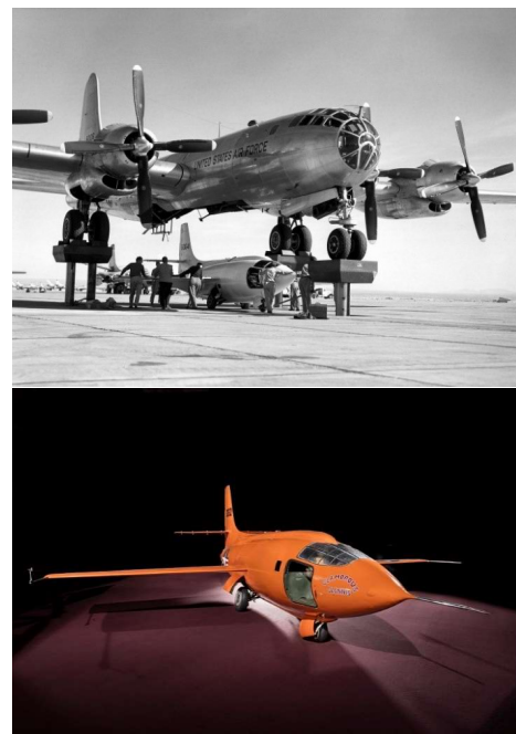
Fig. 21 Bell X-1 preserved in the Smithsonian National Air and Space Museum and being mated to the bomb bay of a B-50. It would be airdropped at a steady speed and altitude.
