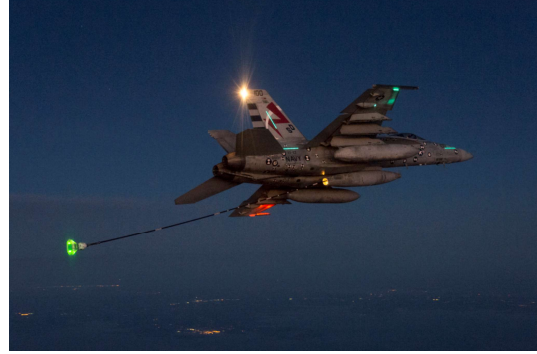
Fig. 14 Static drogue flight instrument calibration testing on an F-18/A. The drogue sags beneath the wake of the aircraft to determine the pressure and temperature of the freestream flow.[38]
