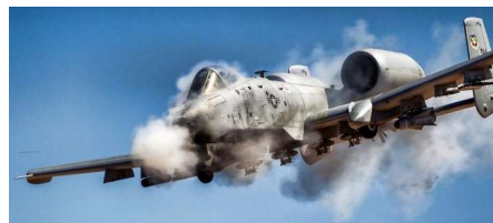
Fig. 8 A-10 Warthog experiencing heavy gun smoke after firing. The smoke erodes the skin and more dangerously can flame out the engines.
