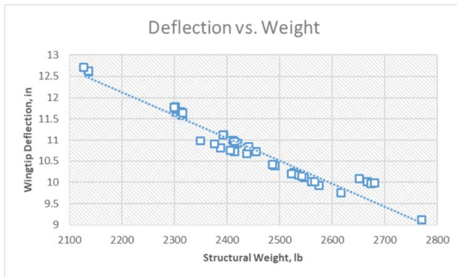
FIGURE 13: Deflection vs Weight - There is a distinct relationship between the structural weight and the stiffness of the wing from a variety of designed wings.
