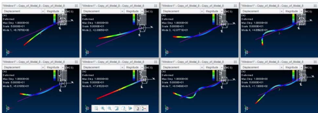
FIGURE 15 – FULL FUEL LOAD MODAL ANALYSIS (HEAVY STRUCTURAL WING)
