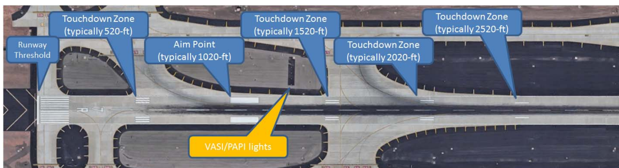
Figure 6 - Runway Markings at KPHX (7R – long runway)
