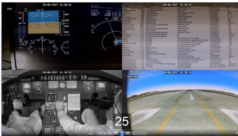
Figure 8 – CRJ-200 Crew Observation Recording Log – PFD, Sim Datalog, Cockpit and external forward view. Spring 2017 – ASU
