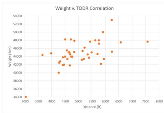
Figure 10 – CRJ-200 All-engines-operating – Take-off-distance to 35-ft ( TODR ) vs dispatch weight. Spring 2017 – ASU
