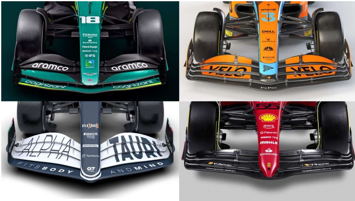
FIGURE 6 - Current Front Wing Designs at Start of Formula 1 2022 Season: a) Aston Martin, b) McLaren, c) Alpha Tauri, d) Ferrari
