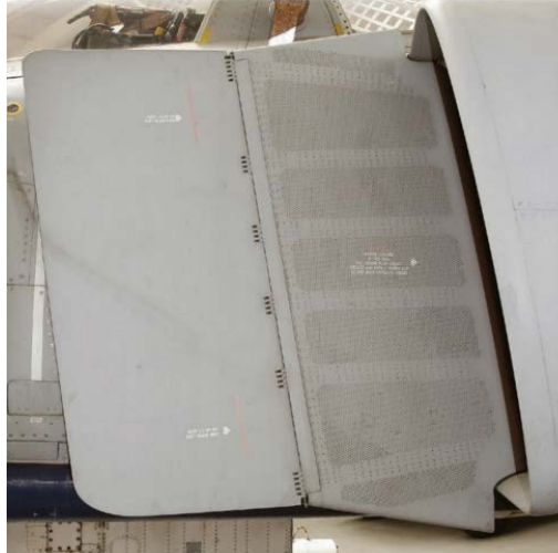
Figure 3 – perforated plate – inlet bleed on external compression ramp of a McDonnell F-4 Phantom
