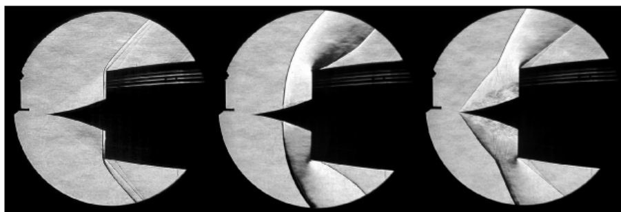
Figure 4 – Schlieren Imaging of an Inlet Experiencing Buzz. (see Ref 16)
