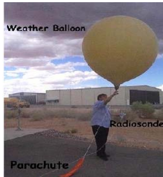
FIGURE 2 - Example NOAA/NWS Radiosonde weather balloon [16]
