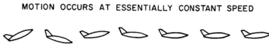
Figure 1 – Short Period Mode Schematic [3]
