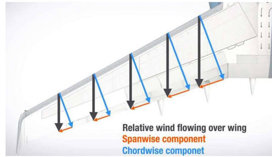
FIGURE 4. Span-wise and Chord-wise Flow Representation on a Swept Wing
