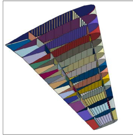
Figure 18. ABAQUS Model With Section Properties
