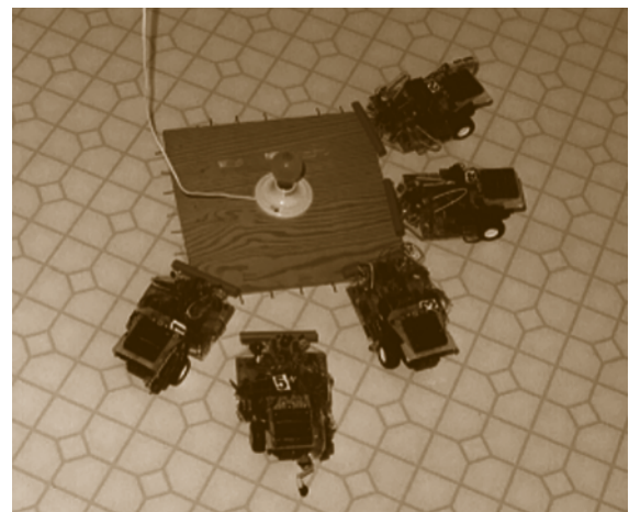
Fig. 72.1 Demonstration of five robots collectively pushing a lighted box (after [72.7])
