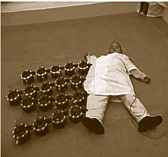
Fig. 72.5 SWARM-BOTS experiment in which s-bots self-assemble to pull a child across the floor (after [72.25])
