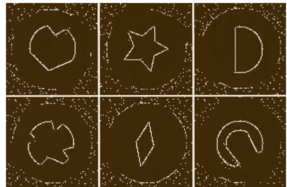
Fig. 72.13 Geometric structures built by a team of 30 robots, in simulation (after [72.48])
