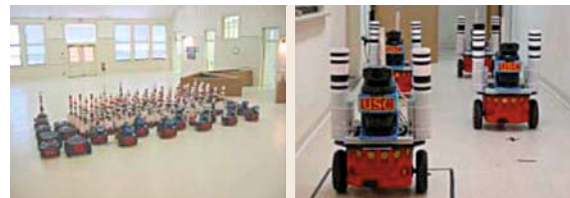
Fig. 41.5 Under the DARPA SDR program, a team from the University of Southern California, the University of Tennessee, and Science Applications and International Corporation (SAIC) demonstrated mapping, and intruder detection by a team of networked robots [41.19]
