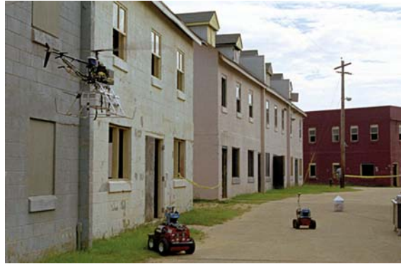
Fig. 40.7 Heterogeneous team of an air and two ground vehicles that can perform cooperative reconnaissance and surveillance
