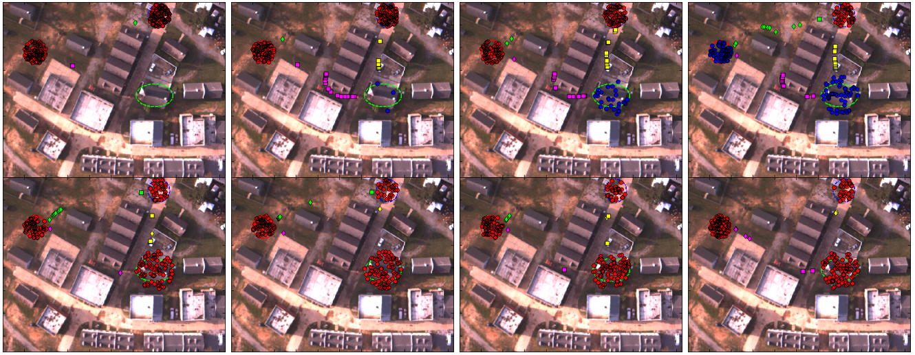
Fig. 6. Snapshots from a simulation redeploying 200 agents, initially located at two sites, to three sites in an urban environment. Agents leaving sites are denoted by square markers and agents entering sites are denoted by diamond-shaped markers. Agents located at sites above quorum are shown in red while agents located at sites below quorum are shown in blue. The system is driven by the model given in ((8)) and taking travel times between sites into account.
